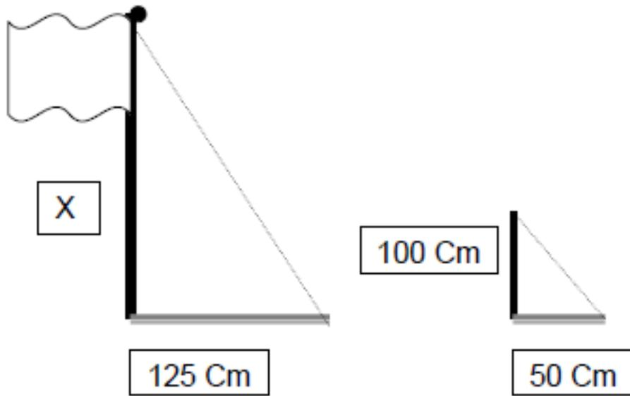
$$\frac{\text{Height of stick}}{\text{Height of flag pole}} = \frac{\text{Meter stick's shadow}}{\text{Flagpole's shadow}}$$
